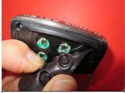
Follow with boot button using your fingers again and applying roll and press movements till catchers of the second button engage with plastic cover. Continue with remaining buttons till all fit tightly in respective holes. Surface of remote should be flat on touch. Any curving will indicate that buttons do not engage properly with the plastic shell.
