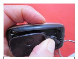
To install your new Silicone pad, you have to push key buttons in respective key holes. You can start with emergency button first and using your fingers, roll and press pad gently till first catchers engage with plastic cover. Do not use any sharp tools as you may damage pad or electronics.
