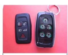
Once plastic skin is peeled or scraped off, you will see key button cut outs and exposed electronic switches. Make sure that surface of the plastic shell is free of any remnants of the old plastic skin.
