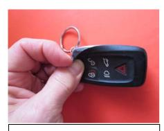
In most cases existing pad is already detached from remote, so you can easily peel it off with your fingers. You can also use flat screw driver to scrape it off.
